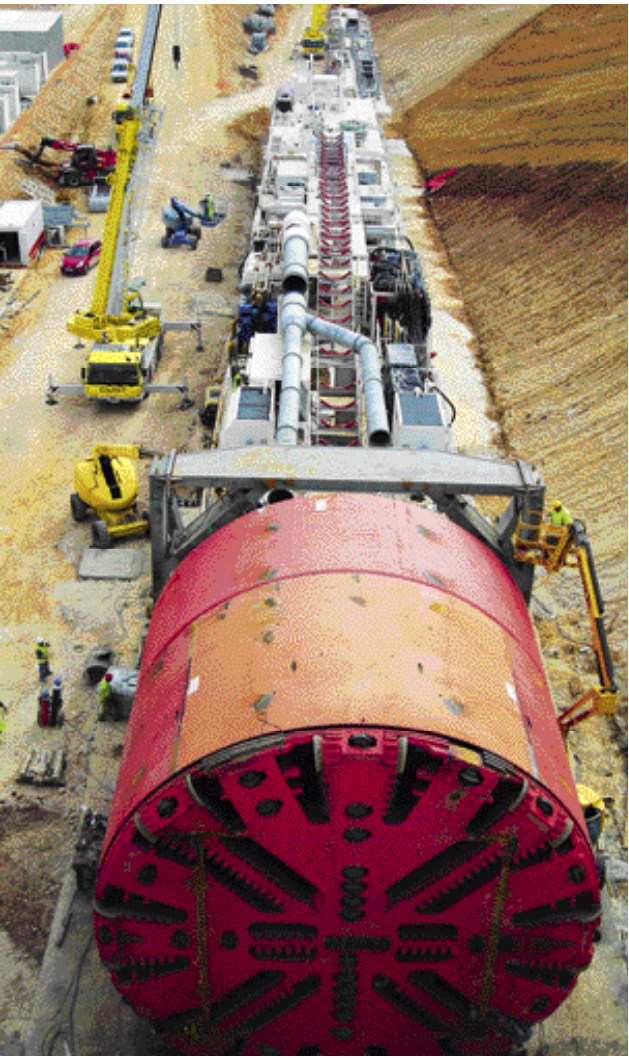
↑ The tunneling machine used in Camarillas has a mixed cutting head.
